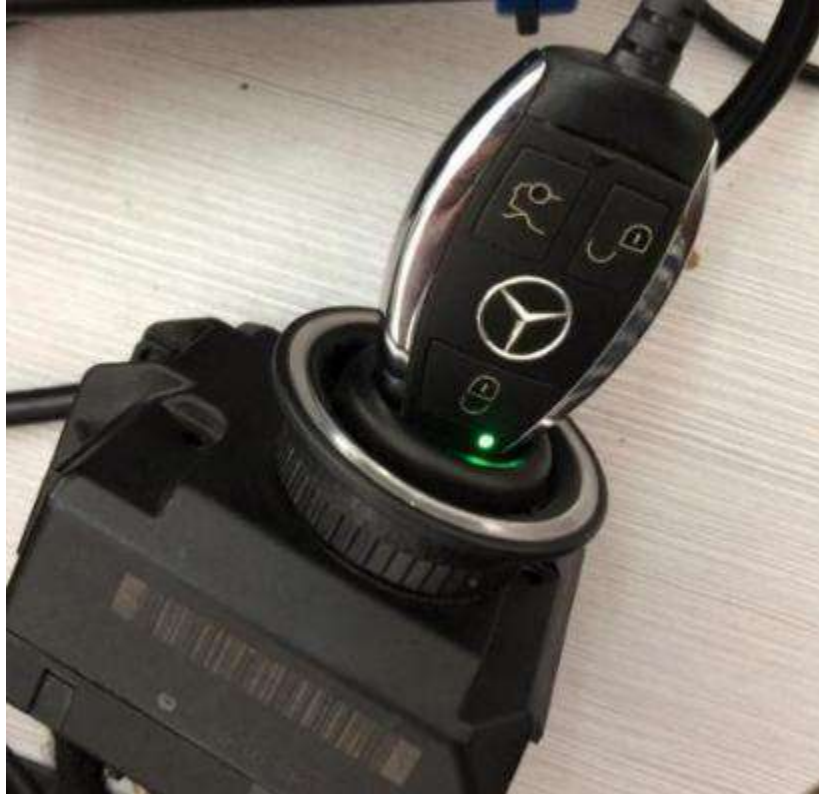
Figure 3.2.4.3 Communicating with EIS/EZS Using the IR Adapter
