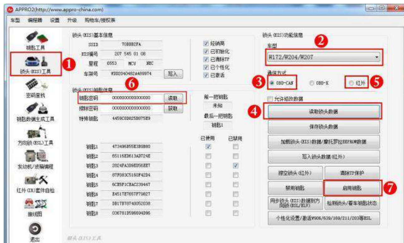
Figure 8.1 Steps for reading the lock status and enabling the key
